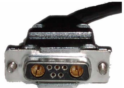
**Figure 4: PWM-CTA Communications Connector**
