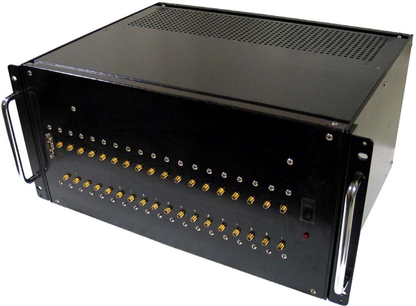
Figure 1: Pulse Width Modulated - Constant Temperature Anemometer
